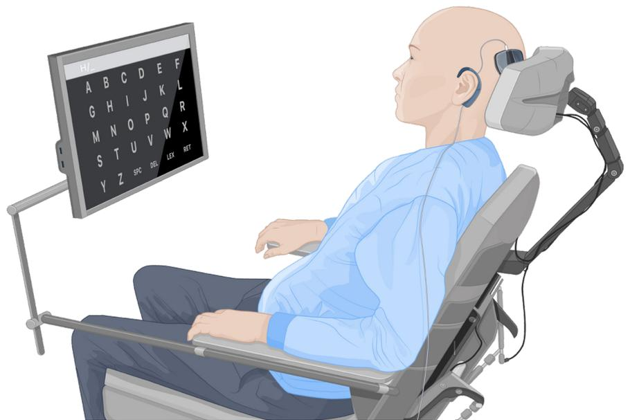
ABILITY: Active Brain Implant Live Information Transfer sYstem. ABILITY is designed for long-term implantation to enable applications such as restoration of communication and movement for people with severe paralysis.
