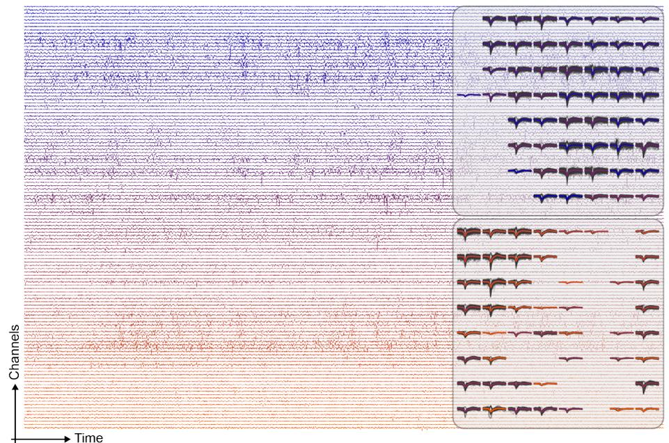
Example of neural data filtered in the spike band, recorded from 128 channels simultaneously over 250 ms. The inserts show locations of channels with action potentials from individual neurons (spikes) on maps of the two electrode arrays. Each spike waveform represents the position of a microelectrode in the array. Not all 128 microelectrode channels show spiking activity in this graphic.
